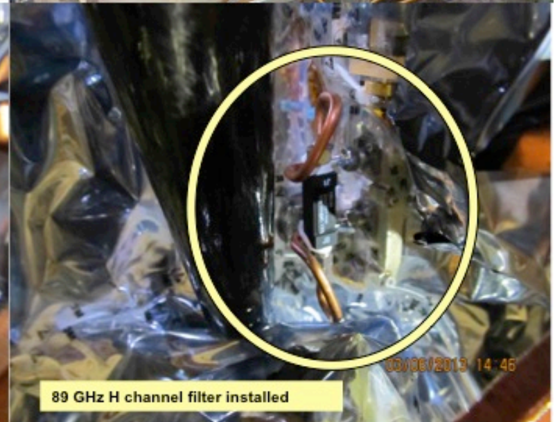
Filter Installation in GMI Clean-room
