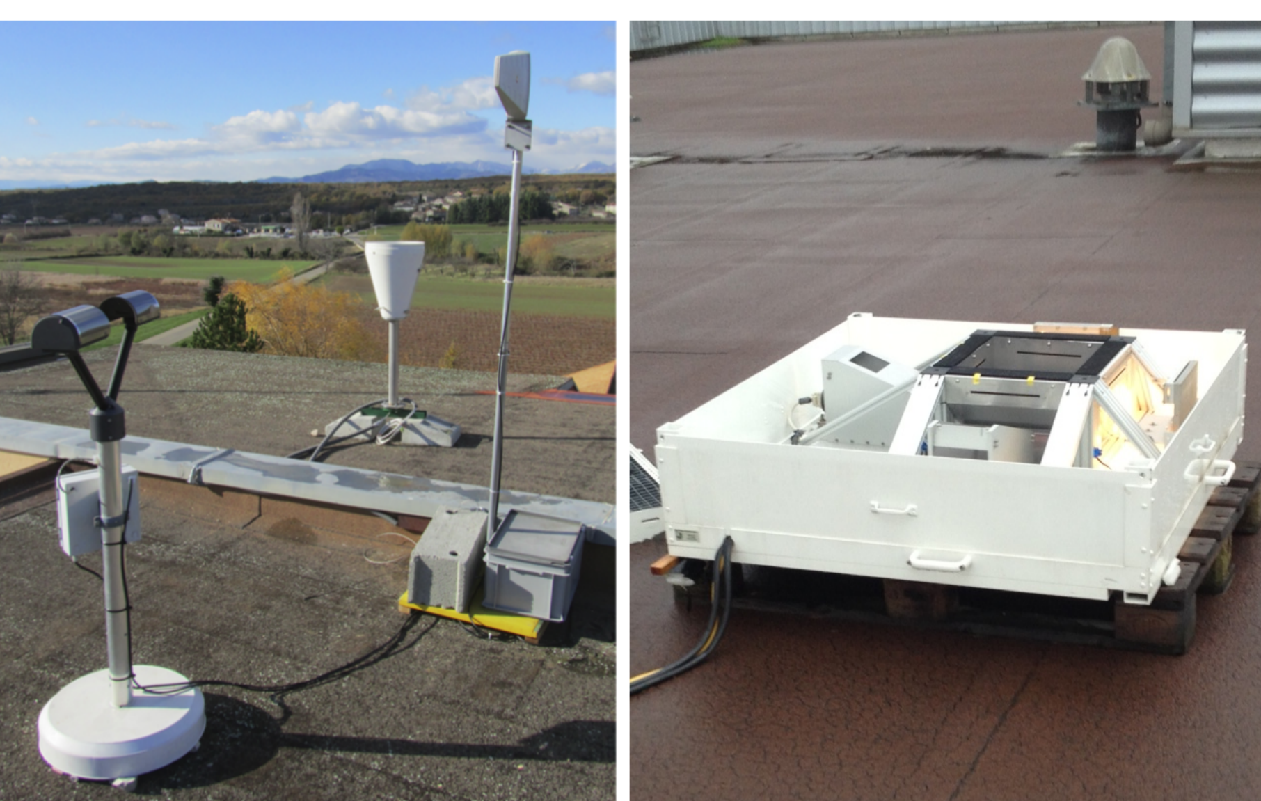
Figure 3: A disdrometer (L) and the 2DVD (R)
