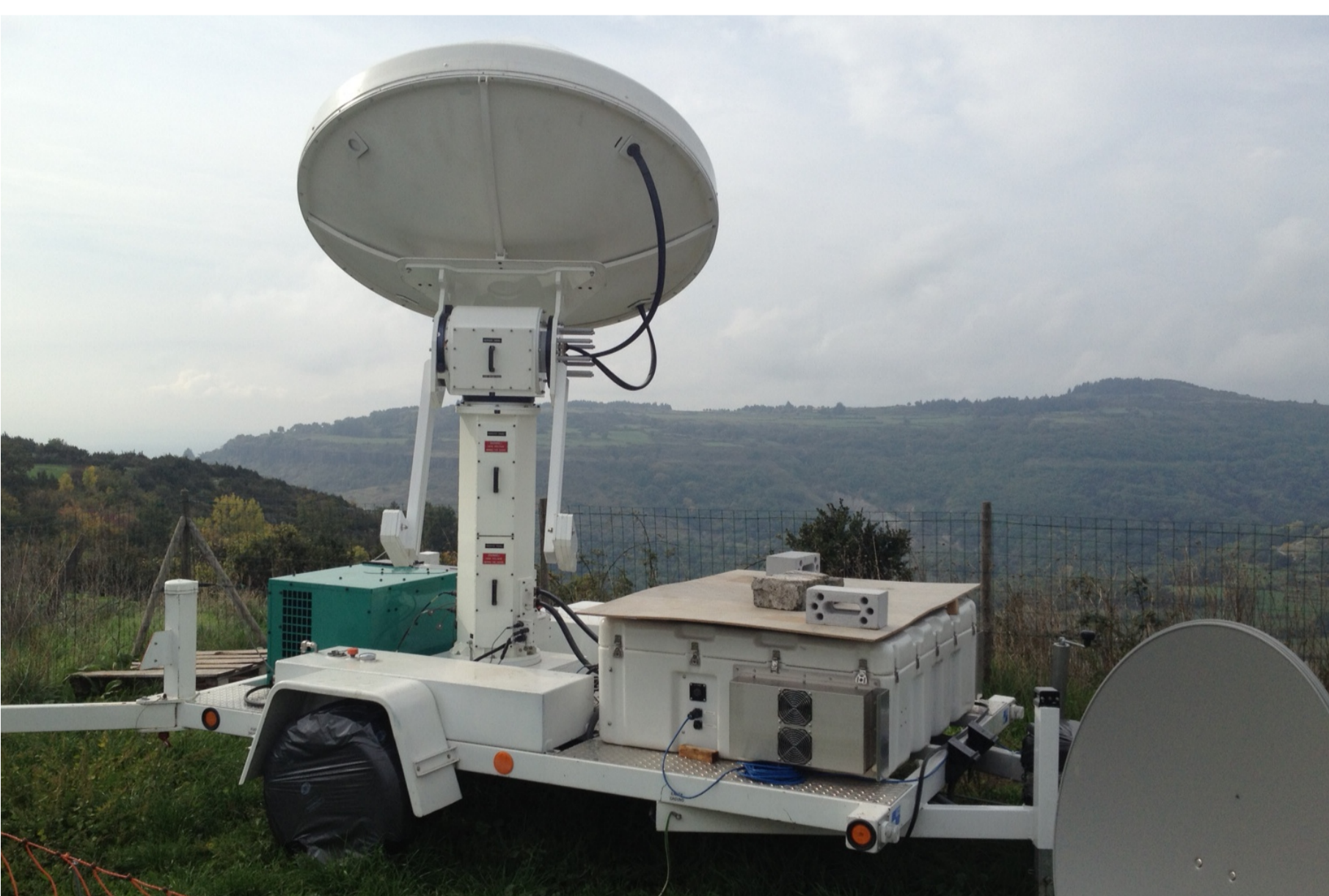
Figure 2: LTE's X-Band radar (MXPol)
