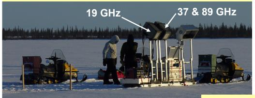
19, 37, and 89 GHz (dual-pol) radiometers will be deployed on a tower for continuous measurements of the surface during the snow cover season.
