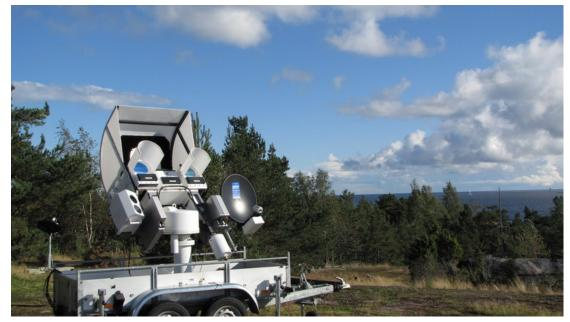
ADvanced Mlcrowave RAdiometer for Rain Identification (ADMIRARI) Dual polarization 10.65 21.0 36.5 GHz (U. Bonn)
