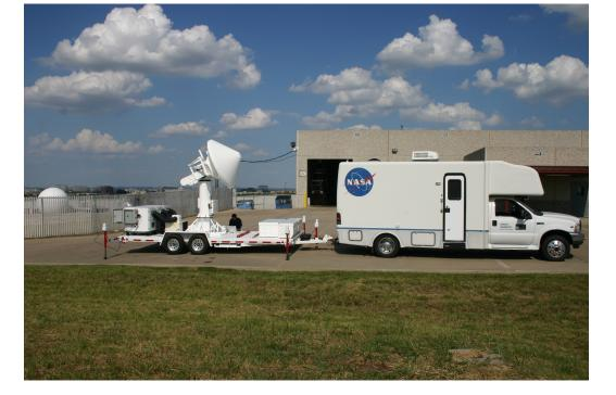
NASA Ka- & Ku-band fully polarimetric, scanning Doppler radar (D3R) • -10 dBZ @ 15 km • 150 m range resolution to 30 km
