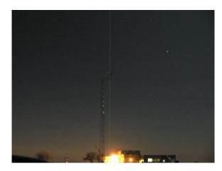
Dual 1064/532 nm polarized lidar
