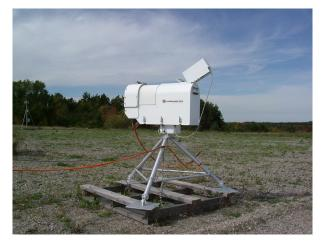
TP3000 profiling radiometer 22 to 30 GHz and 51 to 59 GHz
