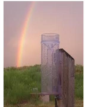
Rain gauges collect rain, or snow, in one spot. By looking at the level of water and reading the measurement mark on the gauge, we can see how much has fallen over a period of time, in a 24-hour day, for example.
