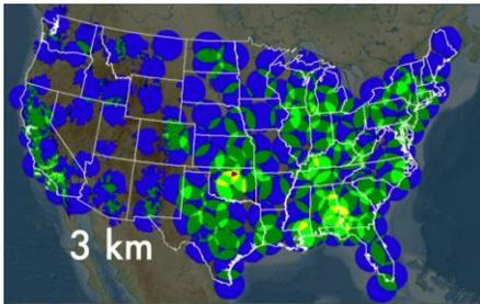
Ground-based radar coverage in the U.S., showing gaps over mountains and limited extent over the oceans.
